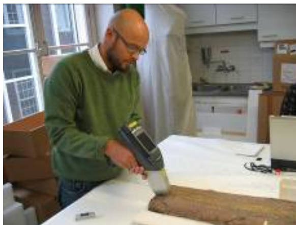
Figure 3: Demonstration of a handheld X-ray fluorescence analyser.
